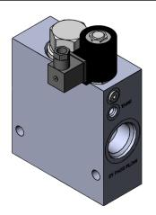
This assembly is design for a maximum input flow of 120 GPM and a maximum priority flow of 50 GPM. To insure proper operation there should be a minimum of 50 PSI pressure at the BYPASS port with or without the solenoid valve actuated. The priority flow is a preset amount that is set when ordered and is not wrench adjustable. This assmbly can be built with different voltage coils on request. For more information call 360-264-2141
