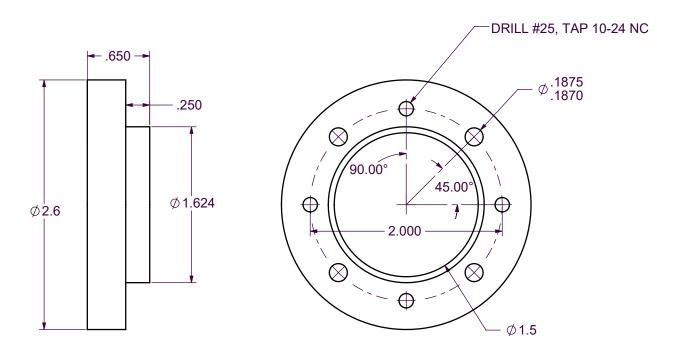
To weld this part to your existing drive gear both parts must be pre heated to a minimum of 200°F or 93°C. Parts should not exceed 800°F or 427°C. If possible use a high strength filler material compatible with 8620 steel. Allow the welded parts to cool slowly. Do not guench in oil or water if above 200°F or 93°C!
